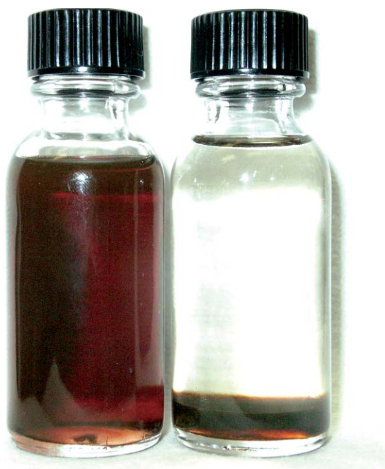
Fig. 4 HFPSA-catalyzed alkylation of xylene in the absence (left) and presence (right) of an ionic liquid.
